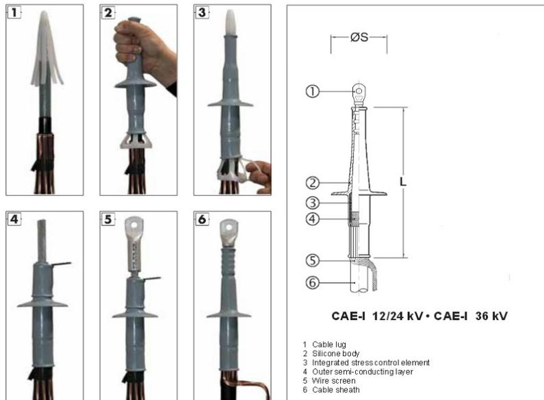
The installation of the termination is practically performed in one quick and easily slip-on step through a patented applicator.
