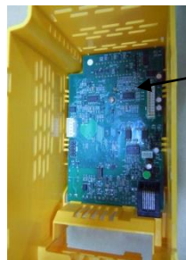
CPU card installed behind the housing
